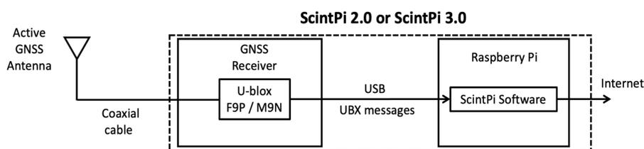
Figure 1 – Main components of our ScintPi 2.0 or ScintPi 3.0 monitors.
