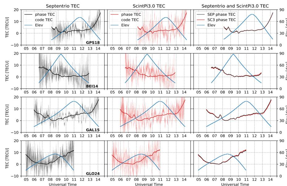
Figure 3 – Collocated ScintPi 3.0 and Septentrio PolaRx5S measurements made at UT Dallas on January 10, 2021.
