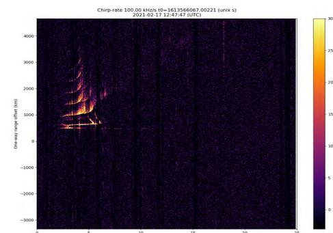
Figure 2. calculated ionogram outputted by the GNU Chirpsounder2 software from a Chirpsounder located in Spring Brook, PA. The chirp signals are transmitted from the ROTHR located in Chesapeake, VA
